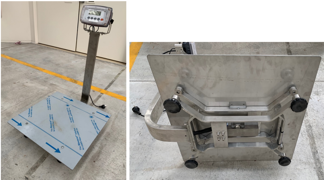
Figure 2 - Model SMS4050-60 (with oversized platter of 600 x 600 mm)
